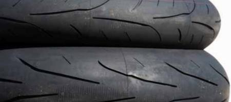
120/70ZR17 180/55ZR17 Ambient: 24 Track: 30 **Stiffness** Front: 58 Shore A Rear: 54 Shore A
